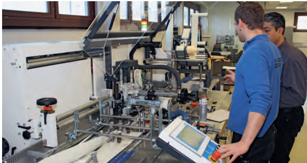
The paper packaging system is based on the "Paper X Hybrid Advance" and has been extended by several units in cooperation with Kohlhammer (see box on page 20). When the system is fully installed, it will measure almost 26 metres in length and can pack much more than just paper.
