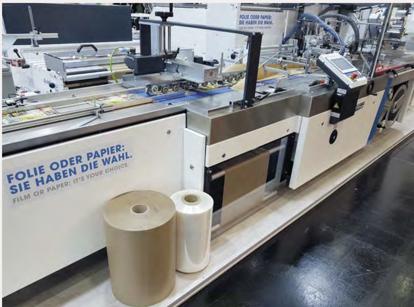
■ Future-proof and flexible: the paper X hybrid advance for film and paper packaging on just one machine. It processes films of all types and papers from approx. 60 g/m 2 to 120 g/m 2 .
